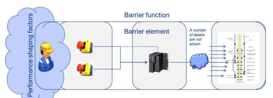
Driller detects a kick and presses one of the available pushbuttons to activate shear ram PLC sets output signals according to the drillers' command
